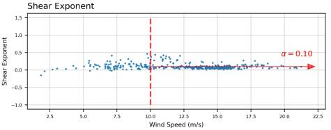
Wind data observed at 86m and 30m heights. Atm. Pressure measured at 20m height.
